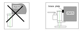
5.4.3 Operators should be very careful to use different jacks to lift a heavy-duty weight. Pay attention to the shifting of center of gravity during lowering or lifting the weight. The total lifting capacity of all jacks should be larger than load of lifted weights. 5.4.4 The owner of jack should guarantee all of the stick labels concerning safety standards keeping on its relative locations, which should be replaced when they can not be read clearly.
