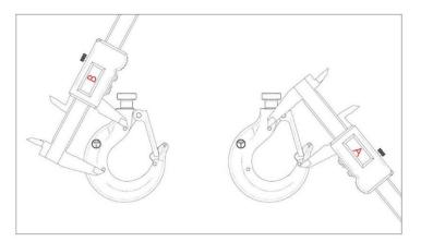
PROLH lever hoists are fitted with the patented Tiger "EZ check" 3 point marking system. With this system a quick check that the A and B measurements are the same (as shown in the diagram below) will indicate if the hooks have stretched If A≦B the hook is fine; If A>B the hook needs to be replaced.
